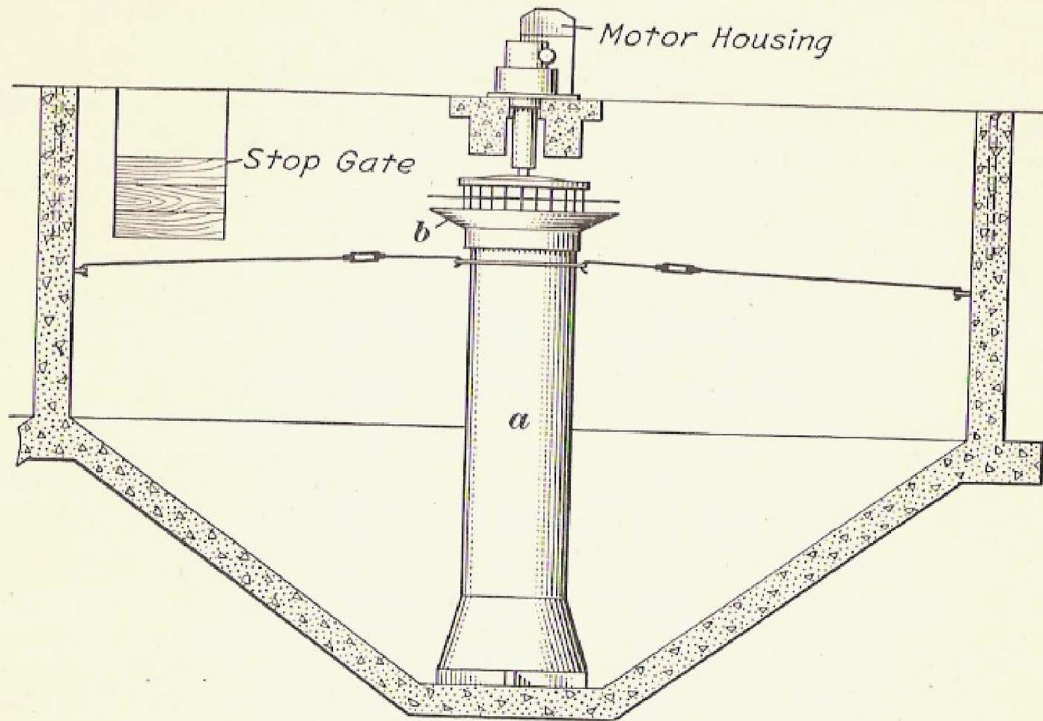
FIG. 117. MECHANICAL AERATOR.
