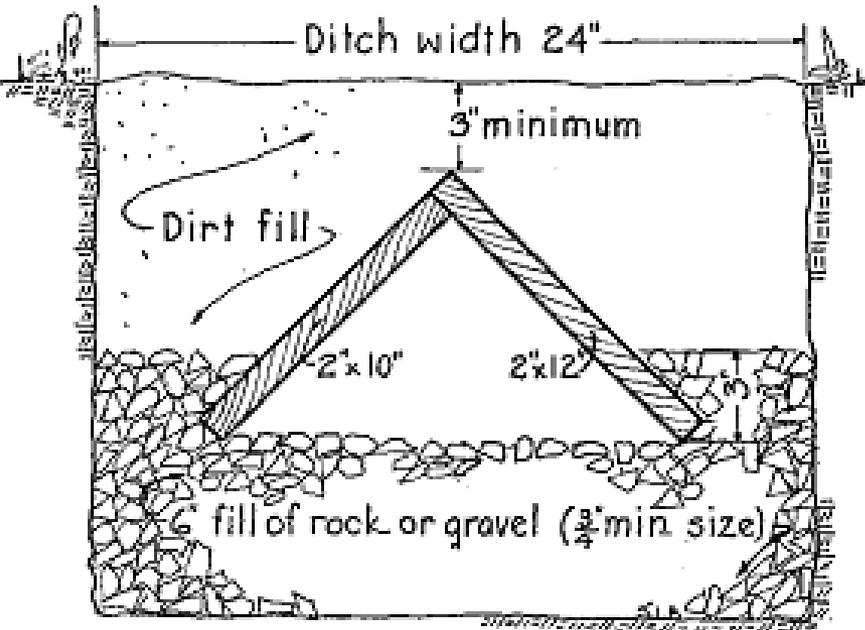
Fig. 14.—Cross section of V-trough drain line.
