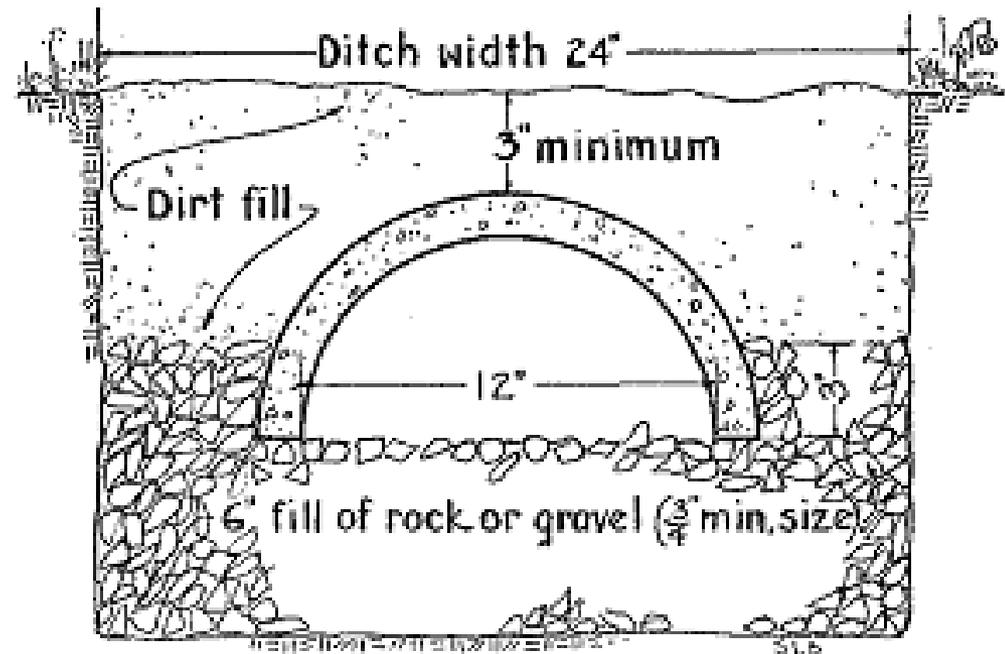
Fig. 16.—Cross section of half-section pipe drain line.
