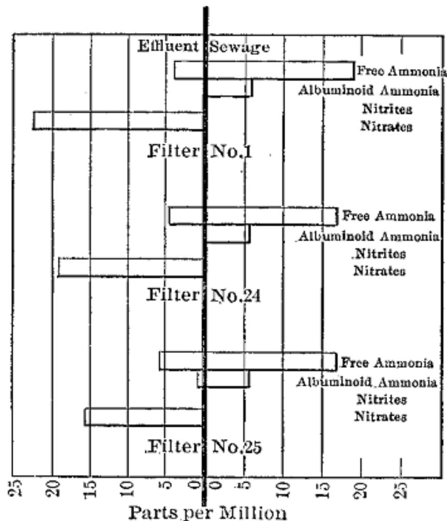
FIG. 65. Nitrogen changes in Intermittent Filtration at the Technology Experiment Station.
