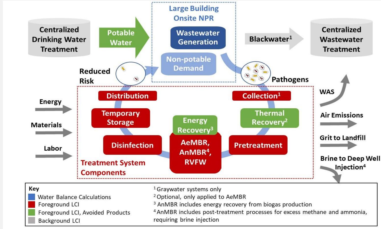
Analyze cost and environmental impact of systems treating mixed wastewater and source separated graywater for onsite NPR (0.01-0.016 MGD). Integrated results with microbial risk assessment.
